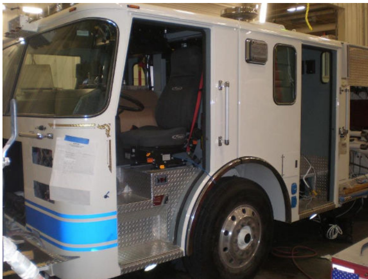
5 Safety upgrades such as new seats and belts, and cabinet reconstruction for rural water tools were all part of the repurposing of this apparatus.
